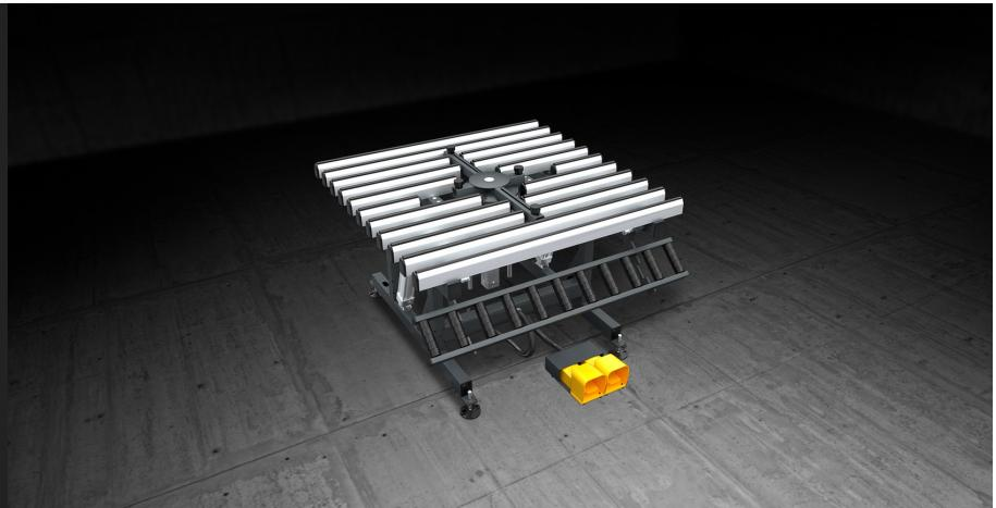
Assembly bench for glazed sashes with work table tilting from 0° (horizontal) to 85°. The drop-away roller conveyor is adjustable in height (from 170 to 460 mm) independently from the work table. The work table is adjustable from 895 to 965 mm while the feet are drilled with holes for floor anchoring. The bench is provided with a central spider clamp for hoisting and positioning the glass.
