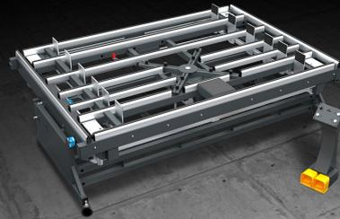
Assembly bench for fitting the aluminium frame with gasket and glazing. The glazing is lifted via a spider clamp and, thanks to a system of self-aligning vices, the frames are pressed two-by-two. After pressing on the first two sides, the spider clamp is rotated and then it is possible to press on the other two sides.
