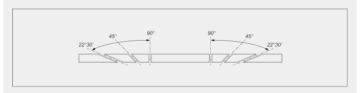
Mechanical adjustment of intermediate angles
