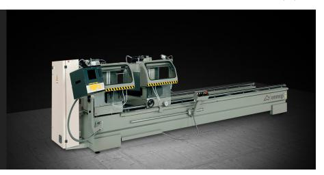
Electronic double-head cutting-off machine with 3 axes for compound cuts. Motorised and electronically controlled rotation of the horizontal axis (22°30′ external and 45° internal) and pneumatic rotation of the vertical axis (45° internal). 500 mm-blade. Available with a useful cut of 4 and 6 m in length.
