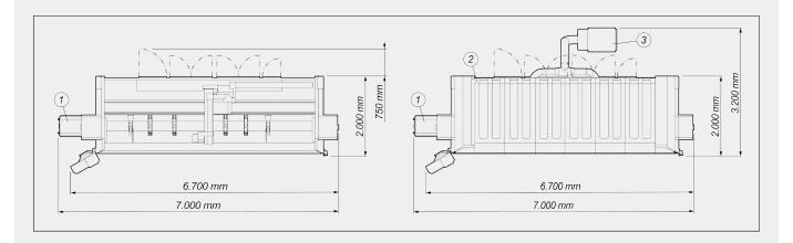
Machine height (maximum Z-axis extension) (mm)
