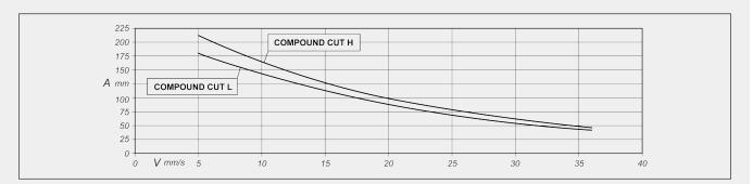
A = contact arc (mm) V = blade feed rate (mm/s)
