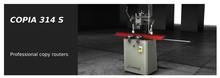
Manual single-head copy router with long vertical travel and traverse of cutting head with handle or indirect lever. Through machining operations can be performed without turning over the workpiece. Manually controlled stylus.
