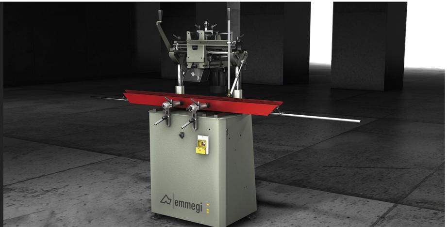
Manual single-head copy router with long vertical travel and traverse of cutting head with handle or indirect lever. Through machining operations can be performed without turning over the workpiece. Manually controlled stylus.
