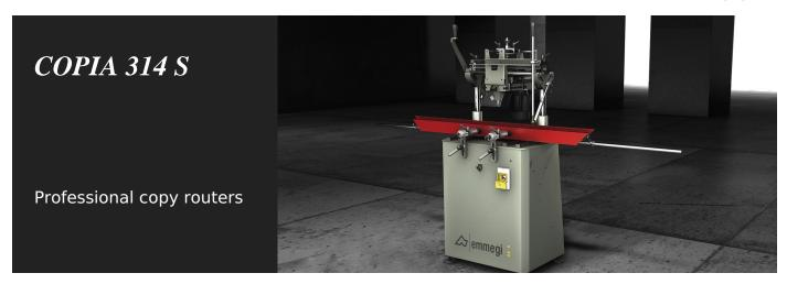
Manual single-head copy router with long vertical travel and traverse of cutting head with handle or indirect lever. Through machining operations can be performed without turning over the workpiece. Manually controlled stylus.
