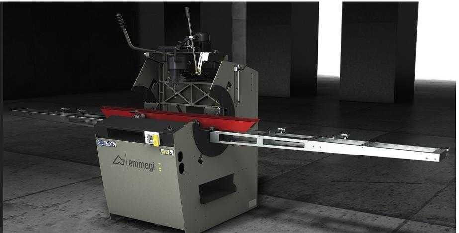
Manually controlled single head copy router with pneumatic clamping and traverse of the head with indirect lever. Ability to run through machining of aluminum without turning the workpiece. Scratch-proof. Manually controlled stylus.
