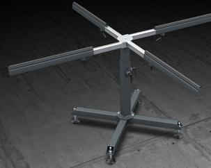
The bench is suitable for accessories and gaskets assembly. It can rotate on a central fulcrum and can be adjustable in length, thus allowing the frame rotation.
