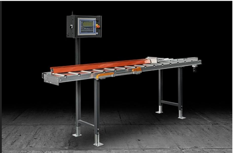
Stop gauge and profile support system with movement of the stop on CN axis and electronic read-out by absolute magnetic band. Equipped with an electronic measurement system that allows to save data on internal memory or transferred in real time to a PC or to the control unit of a miter saw via Bluetooth. It allows machining with high accuracy and repeatability of positioning.
