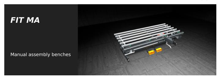
Assembly bench for fitting perimetral band-cut hardware on aluminium, wood and PVC sashes. A system of drop-away vices grips the sash. The bench is equipped with an automatic feeding screwing system and optionally with a system for hardware cutting and measuring with hydro-pneumatic shears.
