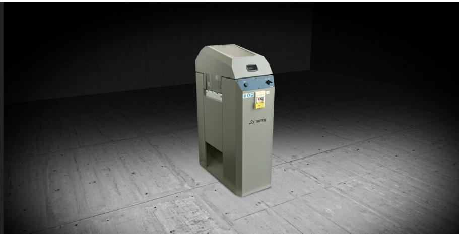
Horizontal end milling machine with manual feed. Mitre milling at 90°. Quick cutter change with manual control. Scratch-proof work table. Full guarding of work zone.
