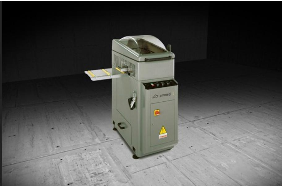
Horizontal end milling machine with electropneumatic feed. Milling of intermediate angles,  $+45^\circ$  /  $90^\circ$  /  $-45^\circ$ . High speed of tool rotation for improved quality machining on painted profiles and at intermediate angles. Quick cutter change with pneumatic control. Scratch-proof work table. Fully guarded work zone with high internal visibility.
