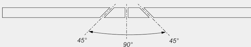
Mechanical adjustment of intermediate angles
