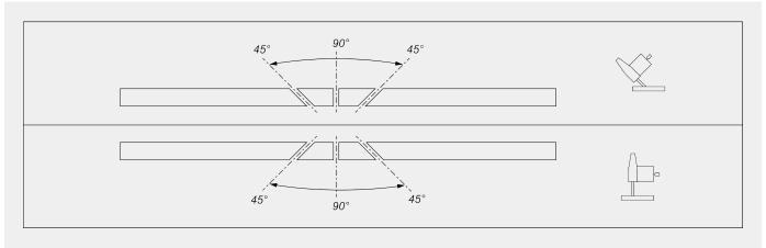
Mechanical adjustment of intermediate angles
