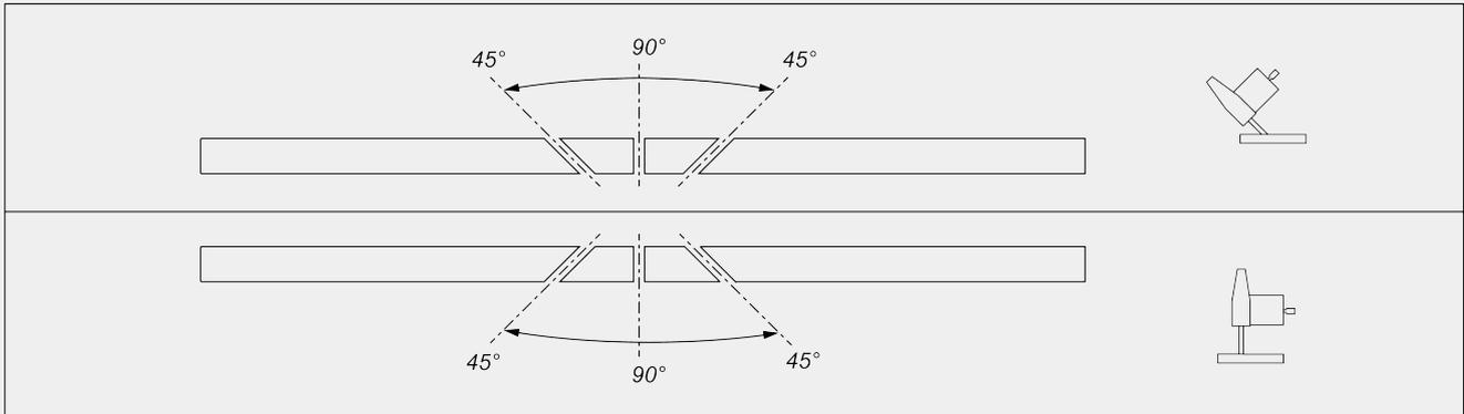
Mechanical adjustment of intermediate angles
