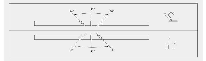
Mechanical adjustment of intermediate angles
