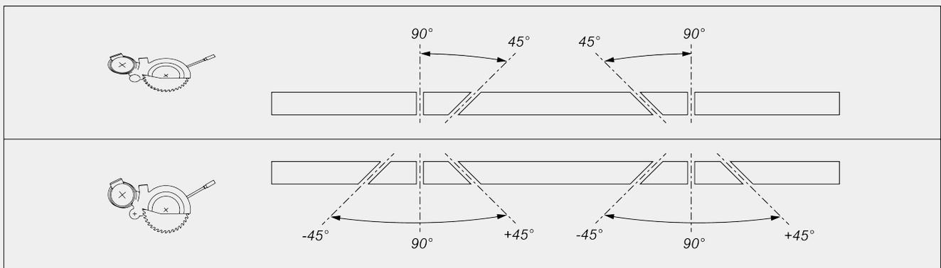
Mechanical adjustment of intermediate angles
