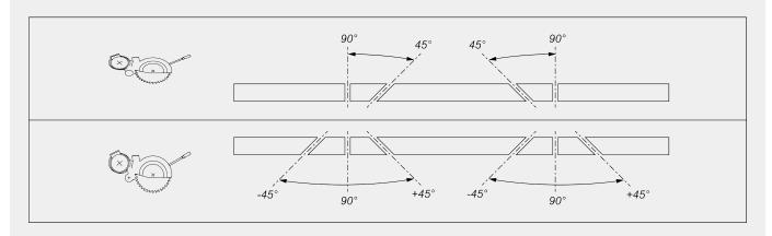
Mechanical adjustment of intermediate angles
