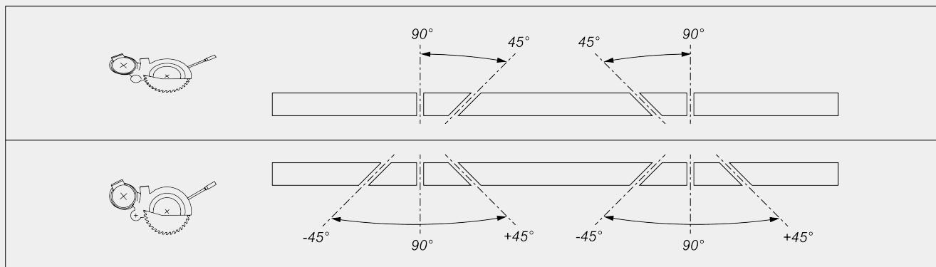
Mechanical adjustment of intermediate angles
