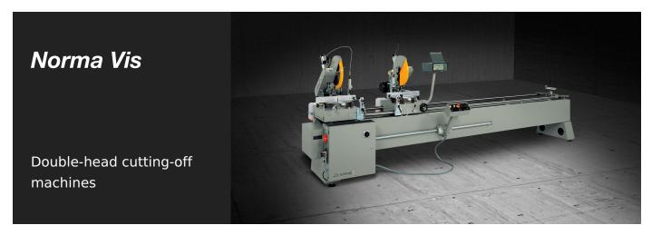
Double-head cutting-off machine with manual movement of the mobile head with digital quota visualizer (Norma Vis). Manual rotation (45° left and right) and tilting (45° in relation to the horizontal axis) of the cutting units. 400 mmblade Available with a useful cut of 4 m or 5 m in length.
