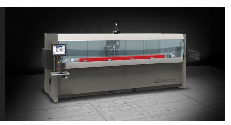
Machining centre CNC with 4 controlled axes, used for working bars of aluminium, PVC, light alloys in general and steel pieces up to 3 mm. It has a 4 tool magazine, with the possibility of hosting 2 angular units and one milling disc. The presence of the rotary work table (CN axis) allows machining at any angle from - 90° to + 90° and on the two heads with a double output angle machining head, with the table at 0°. All CNC axes are absolute and do not require resetting upon machine restart.
