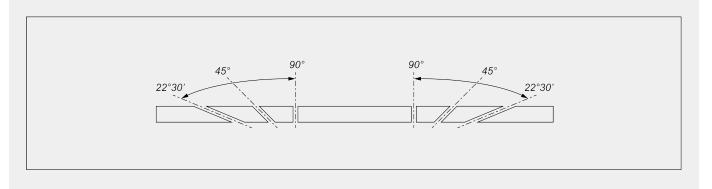
Mechanical adjustment of intermediate angles
