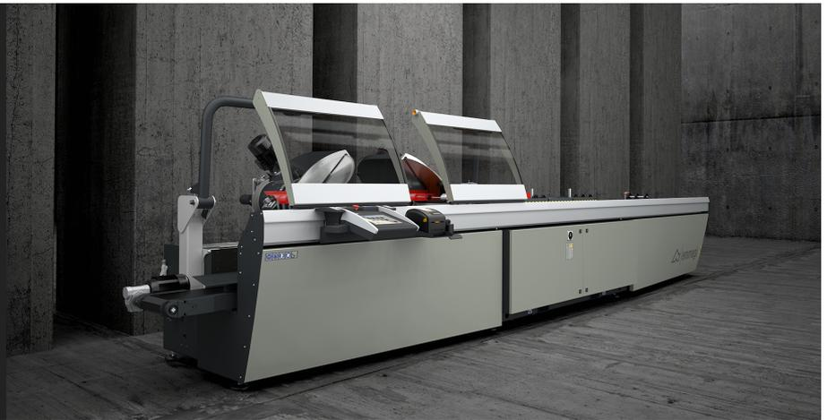
Twin-head cutting-off machine with 3 controlled axes, automatic traverse of the moving cutting head and electronic control of every angular setting from 45° (internal) to 15° (external) with accuracy of 280 places on each degree. The blade feed is controlled by two hydro-pneumatic cylinders.
