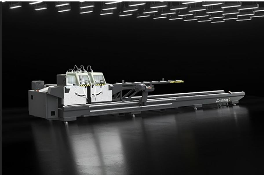
Electronic twin-head cutting-off machine with radial blade movement, automatic traverse of the moving head on recirculating ball bearings by rack and pinion system; tilting inwards up to 30°, designed for cutting large profiles. The blade feed is controled by two hydro-pneumatic cylinders.
