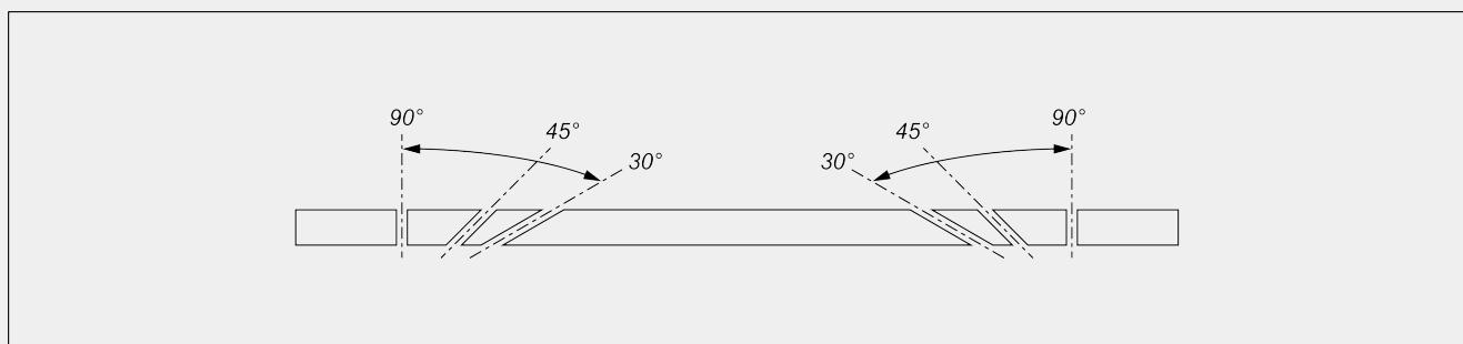
Electronic adjustment of intermediate angles
