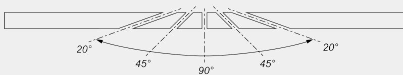
Mechanical adjustment of intermediate angles
