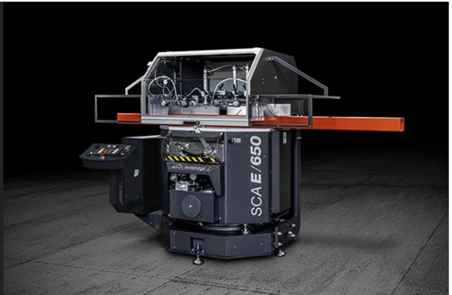
Single-head, rising blade cutting-off machine, with N/C automatic rotation of the vertical axis through brushless motor and contemporaneous hydraulic tilting of the horizontal axis. Cutting with angular settings from 90° to 22°30' (left and right) on the vertical axis and from 90° to 35° (right only) on the horizontal axis.
