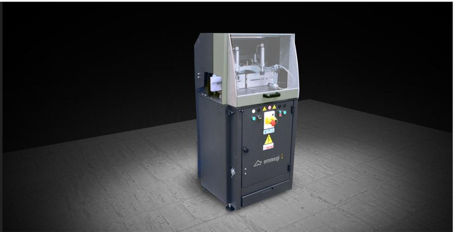
Single-head cutting-off machine with rising blade, with left loading side, able to perform cuts from 15° left to 15° right and intermediate angles.
