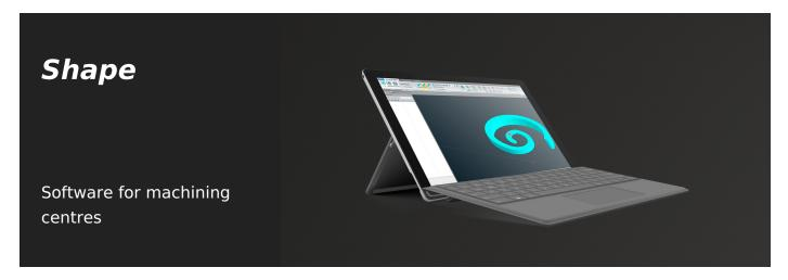
Shape is the software with which you can freely create figures of any shape, freely composing lines, arcs, holes. It is also possible to import figures in DXF format. The 3D display helps better understand the figures at non-constant depths. With Shape, machining operations are now faster than would otherwise be achieved by arranging "standard" figures.
