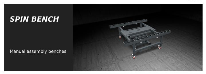
Modular bench for assembly and in-line handling of curtain wall frames. It is provided with two roller tracks covered with soft PVC sheathing; the distance between the two tracks is adjustable according to the width of the curtain wall section. A pneumatically operated system allows clamping the rollers during the work phases. The entire bench can be rotated by 360° in order to facilitate the assembly and sealing of the curtain wall; the angular position is clamped pneumatically.
