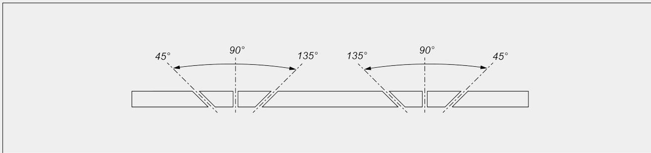
Electronic adjustment of intermediate angles
