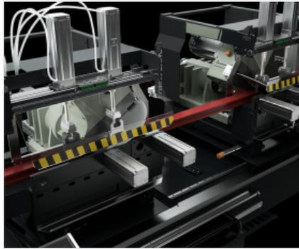
**Internal head inclination up to 150° (Optional)**
