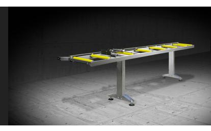
Tubular steel construction with adjustable mounting feet and PVC covered steel rolls. In the version with rolls size 240 mm, roller conveyor length is 3.500 mm; with rolls size 440 mm, roller conveyor length is 4.000 mm.
