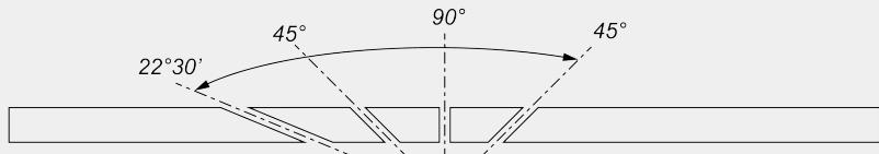
Mechanical adjustment of intermediate angles
