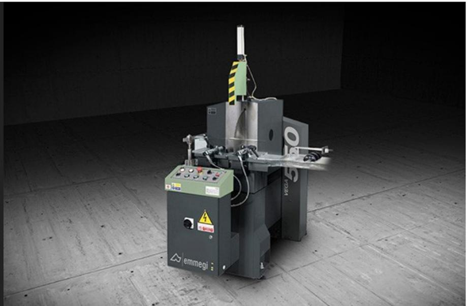
Single-head cutting-off machine with horizontal blade feed and left loading side, pneumatic double side tilting of the cutting head in fixed positions: 45° to the left, 90°, 45° and 22°30' to the right. A special positive stop also allows cutting at intermediate angles.
