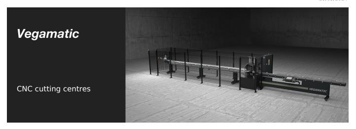
A semiautomatic version cutting centre with 2 controlled axes, manual loading/unloading on opposite sides of the machine, with front CNC blade, dedicated to cutting Aluminium and PVC profiles and light alloys in general. It performs predefined and optimised cutting lists in automatic. Designed to execute cutting at angles ranging from 45° to 135° or from 22°30' to 157°30'
