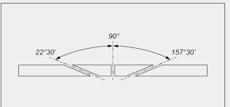
Electronic adjustment of intermediate angles
