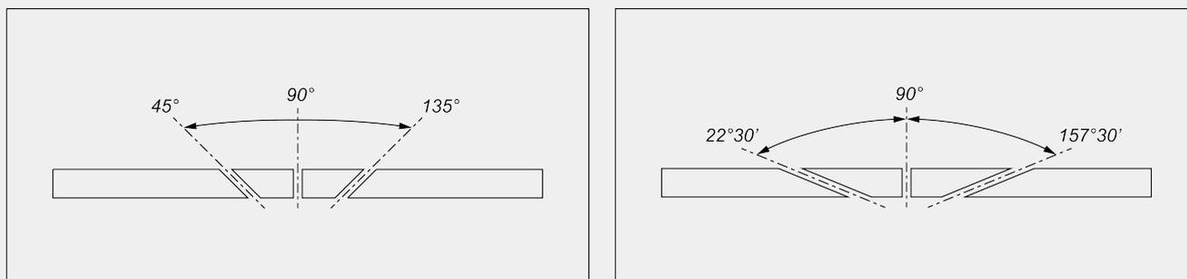
Electronic adjustment of intermediate angles
