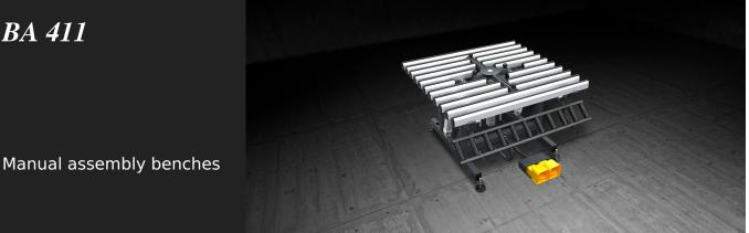
Assembly bench for glazed sashes with work table tilting from 0° (horizontal) to 85°. The drop-away roller conveyor is adjustable in height (from 170 to 460 mm) independently from the work table. The work table is adjustable from 895 to 965 mm while the feet are drilled with holes for floor anchoring. The bench is provided with a central spider clamp for hoisting and positioning the glass.
