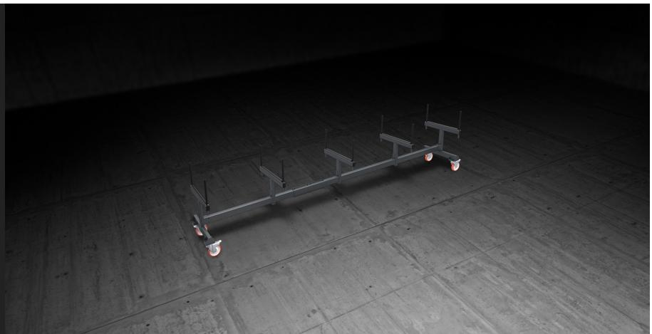
Big size trolley designed for transportation and storage of profiled bars during the cutting phase.
