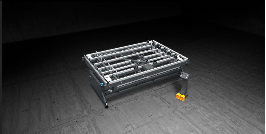
Assembly bench for fitting the aluminium frame with gasket and glazing. The glazing is lifted via a spider clamp and, thanks to a system of self-aligning vices, the frames are pressed two-by-two. After pressing on the first two sides, the spider clamp is rotated and then it is possible to press on the other two sides.
