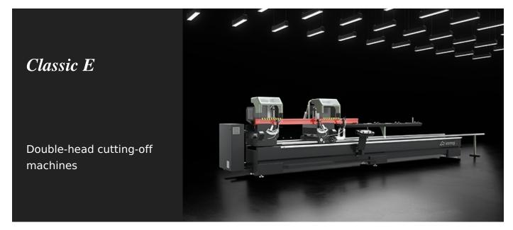
Electronic twin-head cutting-off machine with automatic traverse of the moving cutting head powered by brushless motor with numerical control system. Pneumatic control of the angular setting in three fixed positions 90°, 45° and 22°30' (external) or with mechanic system for manual adjustment of intermediate angles. Hydro-pneumatic blade feed.
