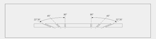
Mechanical adjustment of intermediate angles
