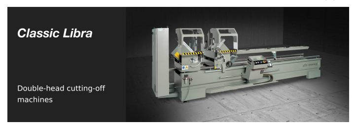
Electronic twin-head cutting-off machine with automatic movement of the head unit using DC motor and pneumatic tilting of the heads outdoors up to 45 ° or 22 ° 30 'depending on the model. Blade 450 and 500 mm. The machine is equipped with electronic meters thickness profile. Available with useful cut of 4,5,6 m in length.
