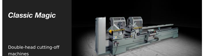
Electronic double-head cutting off machine with automatic movement of the mobile head through a C.C. motor controlled by numerical control. Pneumatic management of all angles up to 22°30′ (external). 450 and 500 mm-blade. Available with a useful cut of 4, 5, 6 m in length.
