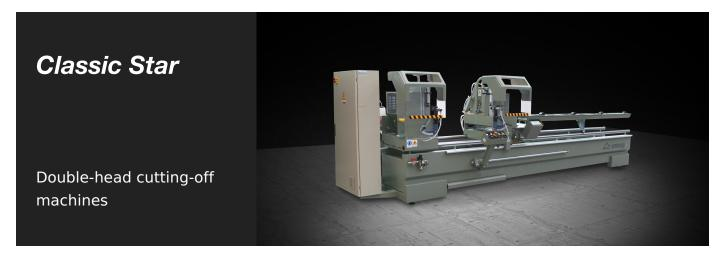
Electronic double-head cutting off machine with automatic movement of the mobile head through a C.C. motor and outward pneumatic tilting of the heads up to 45° or 22°30′, according to the model. 450 or 500 mm-blade. Equipped with an industrial computer for an optimal viewing of the cutting lists. Available with a useful cut of 4, 5, 6 m in length.
