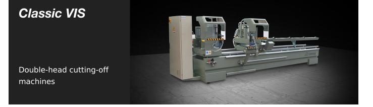
Double head cutting-off machine with manual movement of the mobile head and parameter reading through digital display screen. Outward pneumatic tilting of the head up to 45° or 22°30' depending on the model. 450 and 500 mmblade. Available with a useful cut of 4, 5, 6 m in length.
