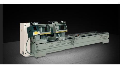
Electronic double-head cutting-off machine with 5 axes for compound cuts. Motorised and electronically controlled rotation of the horizontal axis (22°30′ external and 45° internal) and the vertical axis (45° internal). 500 mm-blade Available with a useful cut of 4 and 6 m in length.
