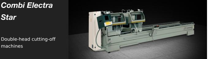
Electronic double-head cutting-off machine with 3 axes for compound cuts. Motorised and electronically controlled rotation of the horizontal axis (22°30' external and 45° internal) and pneumatic rotation of the vertical axis (45° internal). 500 mm-blade. Available with a useful cut of 4 and 6 m in length.
