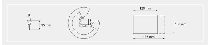
Maximum machinable section on 4 sides - L x H (mm)120 x 100Maximum machinable section (partially) on the upper face - L x H (mm)185 x 100Y-axis machinable width on the upper face (mm)120
