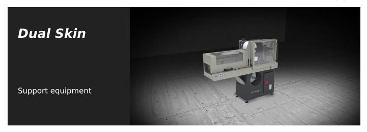
Machine for application of protective film on aluminium profiles. The profile is fed automatically via motorized rolls while the perfect adhesion of the film to the profile is ensured by pressure rolls. An optional additional kit allows applying the film simultaneously also on a third face.
