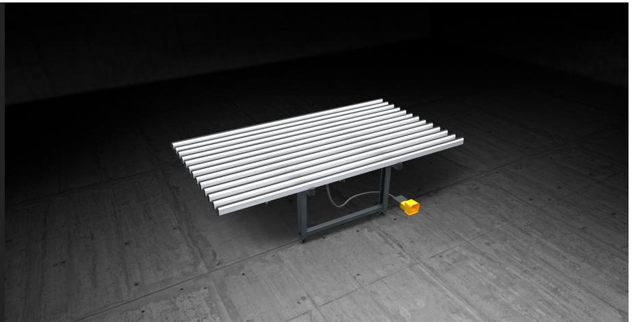
Sash and casement assembly bench. Horizontal bench with pneumatic exchange between the soft PVC resting surface (for assembly operations) and the anti-friction hard PVC resting surface (for handling operations). The work table height is adjustable from 895 to 965 mm and the mounting feet are complete with holes for floor anchoring.
