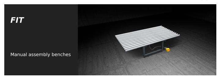
Sash and casement assembly bench. Horizontal bench with pneumatic exchange between the soft PVC resting surface (for assembly operations) and the anti-friction hard PVC resting surface (for handling operations). The work table height is adjustable from 895 to 965 mm and the mounting feet are complete with holes for floor anchoring.
