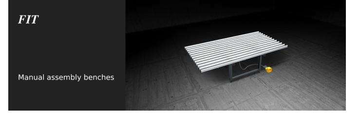
Sash and casement assembly bench. Horizontal bench with pneumatic exchange between the soft PVC resting surface (for assembly operations) and the anti-friction hard PVC resting surface (for handling operations). The work table height is adjustable from 895 to 965 mm and the mounting feet are complete with holes for floor anchoring.
