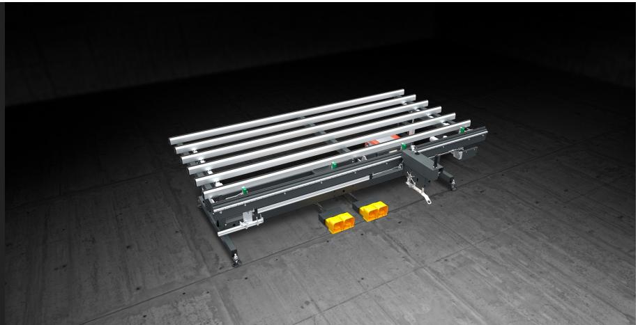
Assembly bench for fitting perimetral band-cut hardware on aluminium, wood and PVC sashes. A system of drop-away vices grips the sash. The bench is equipped with an automatic feeding screwing system and optionally with a system for hardware cutting and measuring with hydro-pneumatic shears.
