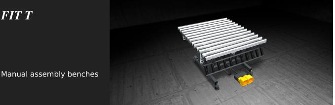
Sash and casement assembly bench. Tilting table from 0° (horizontal) to 85°, with pneumatic exchange between the soft PVC resting surface (for assembly operations) and the anti-friction hard PVC resting surface (for handling operations). The roller conveyor can be manually tilted and it is adjustable in height (from 170 to 460 mm) independently from the work table height. The work table height is adjustable from 895 to 965 mm and the mounting feet are complete with holes for floor anchoring.
