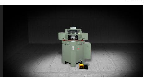
The machine has two special operating heads equipped with masses in which the 2 knives are adjustable on all crimping positions. The knives move and are adjustable on the Y axis (along the profile), on the Z axis (top-bottom) and on the X axis (along the crimping direction). These conditions prevent the replacement of tools on the machine regardless of the different types of profiles. In this way, the times and costs of placing are reduced.
