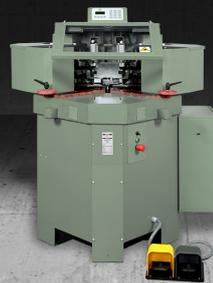
The machine has two special operating heads equipped with masses in which the 2 knives are adjustable on all crimping positions. The knives move and are adjustable on the Y axis (along the profile), on the Z axis (top-bottom) and on the X axis (along the crimping direction). These conditions prevent the replacement of tools on the machine regardless of the different types of profiles. In this way, the times and costs of placing are reduced.
