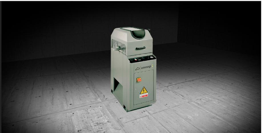
Horizontal end milling machine with manual feed. Milling of intermediate angles,  $+45^\circ / 90^\circ / -45^\circ$ . Quick cutter change with pneumatic control. Scratch-proof work table. Fully guarded work zone.
