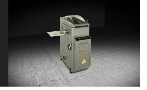
Horizontal end milling machine with electropneumatic feed. Milling of intermediate angles, +45° / 90° / -45°. High speed of tool rotation for improved quality machining on painted profiles and at intermediate angles. Quick cutter change with pneumatic control. Scratch-proof work table. Fully guarded work zone with high internal visibility.
